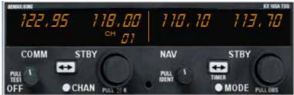
The Bendix KX 165A Nav Com radio has four knobs and four buttons. Its display is divided in two segments. The left portion of the digital display readout is allocated for COMM ACTIVE and COMM STANDBY frequencies channels stored (this is a dummy function in this version). The right portion of the display is allocated to NAV receiver information and much more as shown below.
