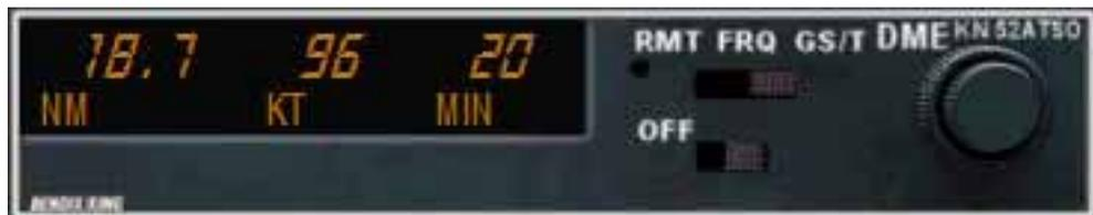
Finally, place the function switch in the Remote (RMT) position, and your DME will be channeled when you select your NAV frequency on the NAV receiver. When the unit locks on a ground station, it will display distance, groundspeed and time-to-station. Note that you may have two frequencies available at all times (one remotely selected on the NAV receiver and one internally selected with the unit's controls).
