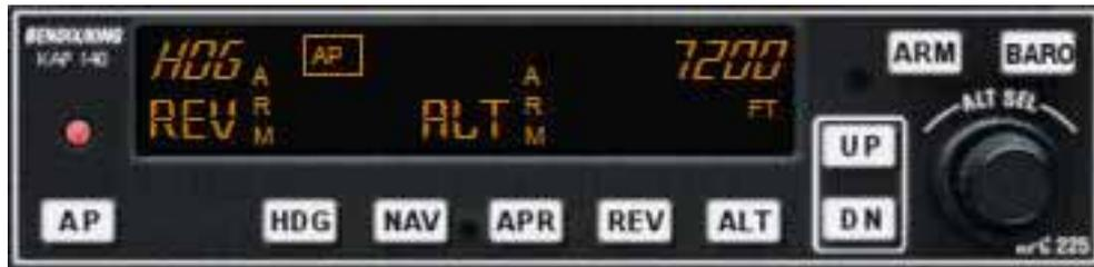
The Bendix KFC 225 AUTOPILOT has one knob and twelve buttons (ten for the KAP 140). Most of functions are the same in both gauges.
