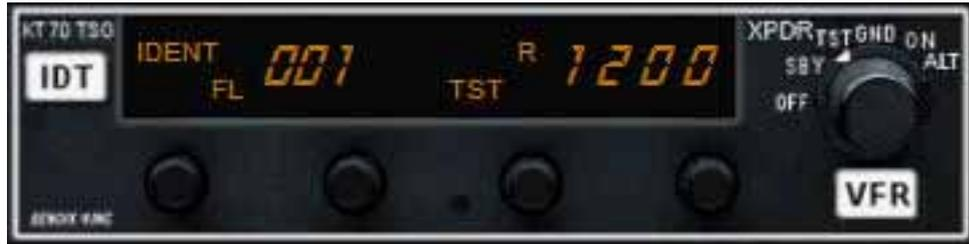
The Bendix KT 70 Transponder has five knob and two buttons. The four little knobs are for setting xpndr code and the big one to select mode.
