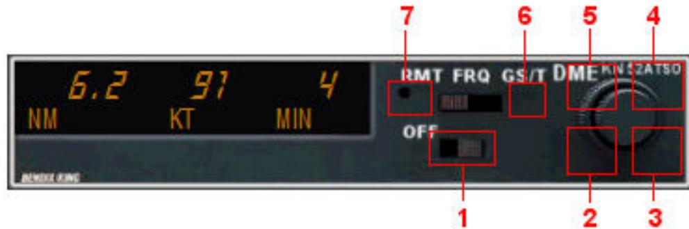
The Bendix KN 62A DME has one knob and two switches. The 3-position function switch determines both, the information displayed and the channeling source.
