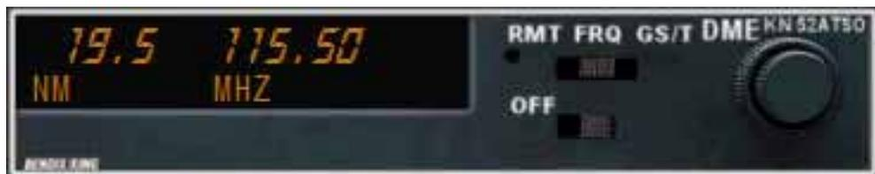
If you move the function switch to the Groundspeed/Time-to-Station (GS/T) position, the unit will hold the internally selected frequency and will display distance, groundspeed and time-to-station. Acting on frequency selector will have no effect on the display, because the DME is in "Frequency Hold". This frequency hold feature in the GS/T mode prevents accidental rechanneling of the DME when the frequency is not displayed.
