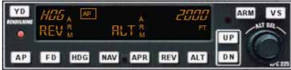
The Bendix KFC 225 AUTOPILOT has one knob and twelve buttons.
