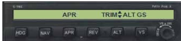
The **ALT** annunciator remains on. Glide-slope capture is indicated by extinguishing of the **ALT** annunciation.
