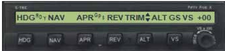
The System Fifty Five X is a rate autopilot that controls the roll and pitch axes of the aircraft. As the pilot enters the desired mode by pressing the appropriate mode selector switch, the computer acknowledges the mode, causing the appropriate annunciator to illuminate.
