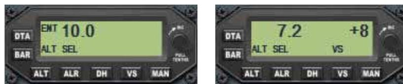
**NOTE:** In entry mode, only the altitude select mode annunciator will be active when “ALT” is selected - the actual altitude can not be called up to the display.
