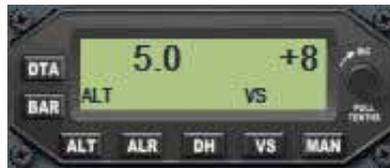
The vertical speed display is the only function that can be accessed directly in the operate mode, therefore, vertical speed changes can be commanded by simply rotating the selector knob. If you are in the “Entry” (ENT) mode you can access the VS Mode by selecting the VS button and then rotating the selector for the desired vertical speed. Pushing VS while in operate mode will hide/display de vertical speed selected.
