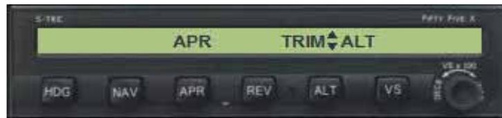
Glide-slope arming will occur when Glide-slope signal be valid. Illumination of the **GS** annunciator will occur, indicating arming has been accomplished.
