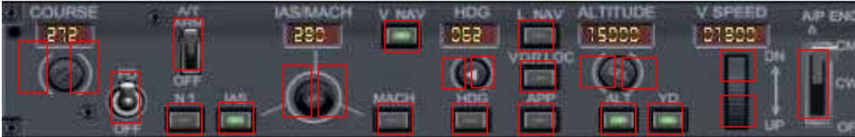
Please, note that the VNAV button only works if FMC-CDU has been properly activated. LNAV button will make the aircraft follow the flight plan route (if any) anytime you press it. It has nothing to do with FMC.
