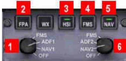
Knobs 1 and 6 select what is driving blue and white needles in PFD. The option selected is shown in the PFD lower display:
