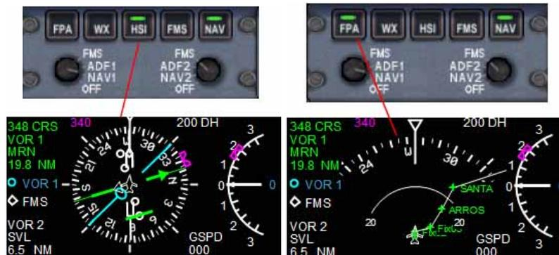
Buttons 4 and 5 change between FMC(4) navigation and normal(5) navigation. To follow FMC navigation (flight plan) you have to activate LNAV button in autopilot too.
