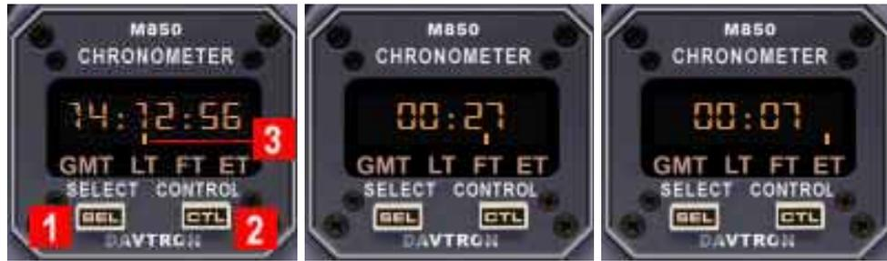
The SEL button(1) selects what is to be displayed, and the CTL button(2) controls the timers.
