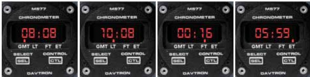
FT starts counting when a valid groundspeed was first greater than 30 knots (typically during takeoff) and it will stop when that speed come down to less than 30 knots. ET starts counting when you click on control button while ET is selected (the red dot is above ET)
