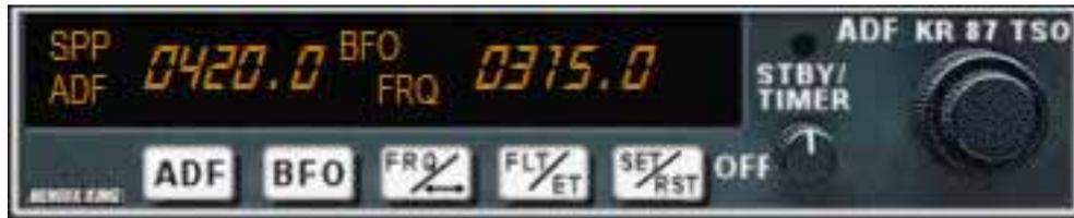
The Bendix KR 87 ADF has two knobs and five buttons. It displays active and stand by frequencies and integrates two timers.
